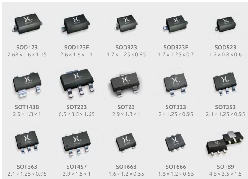
Figure 92 | Table of Nexperia diode leaded-packages with outline and dimensions in mm.
